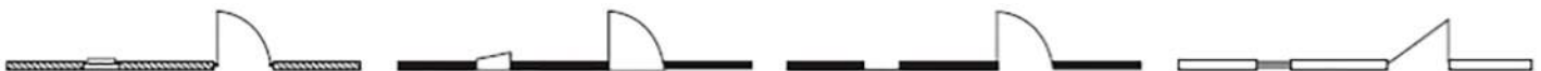
Fig 1. Different ways to draw a wall with a window and a door. The variable graphic symbols pose challenges for automatically recognition of objects in CAD drawings [12].
