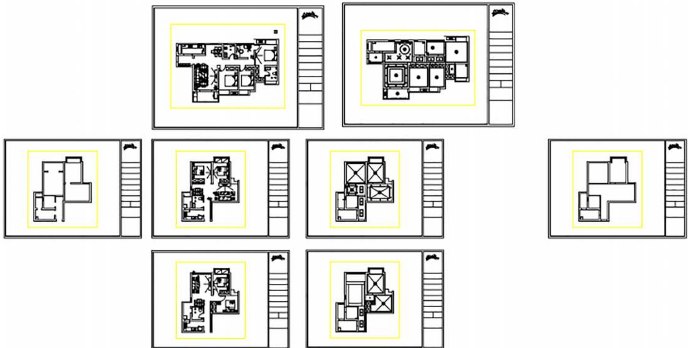
Fig 3. An example of multiple floor plans in a single CAD drawing; systematic clustering is employed to classify lines based on Euler distance.
