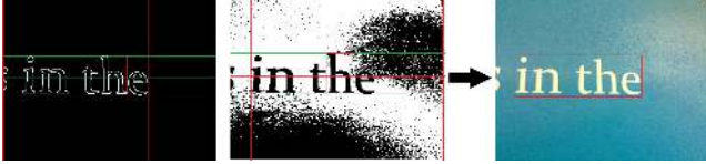
Figure 8. Considering only information from edges (left) or intensity (middle) can determine an incorrect bounding box. Combining both features produces a better bounding box (right).
