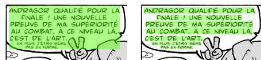
Figure 9: Ground truth bounding boxes (translucent green rectangles overlapping text) at paragraph level (left part) which overlap graphic elements at the bottom-right part and blank areas at the extremities of lines. At line level (right part) which is a lot more accurate than paragraph level. Sources: (Cyb, 2009).
