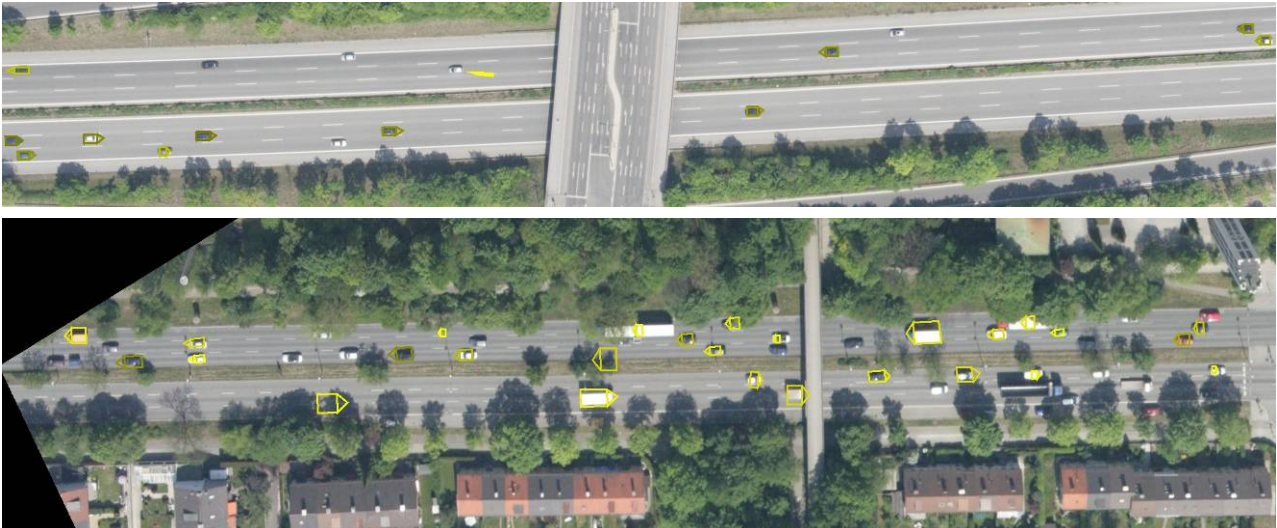
Figure 6. Examples for vehicle detection on motorways (upper image, A96 exit Munich-Blumenau, clipped nadir exposure) and in the city (lower image, Munich “Mittlerer Ring”, clipped side-look-left exposure). Rectangles mark automatic vehicle detections, triangles point into direction of travel.
