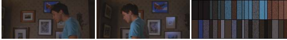
Figure 5: Results: learnt occlusion edge models. Sampling pixels from either side of the T-junctions detected in the input sequence (left and middle) produces the GMM occlusion edge model shown on the right. Each column is a single 6D Gaussian with the first row sampled from the foreground marginal and the second row sampled from the background marginal. The width of each column is proportional to the mixing coefficient of that Gaussian.
