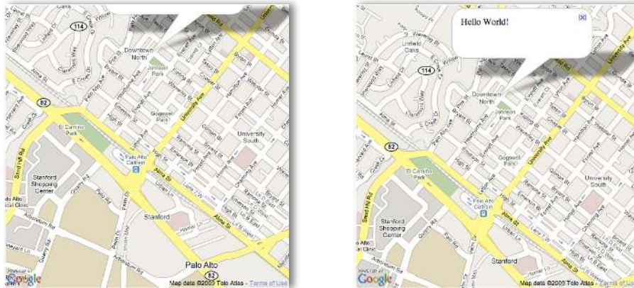
Fig. 2. Issue 519 of the Google Maps API, the faulty behavior on the left hand side is obtained by executing SEQ1a of Figure 1; the correct behavior on the right hand side is obtained by executing SEQ1b of Figure 1.
