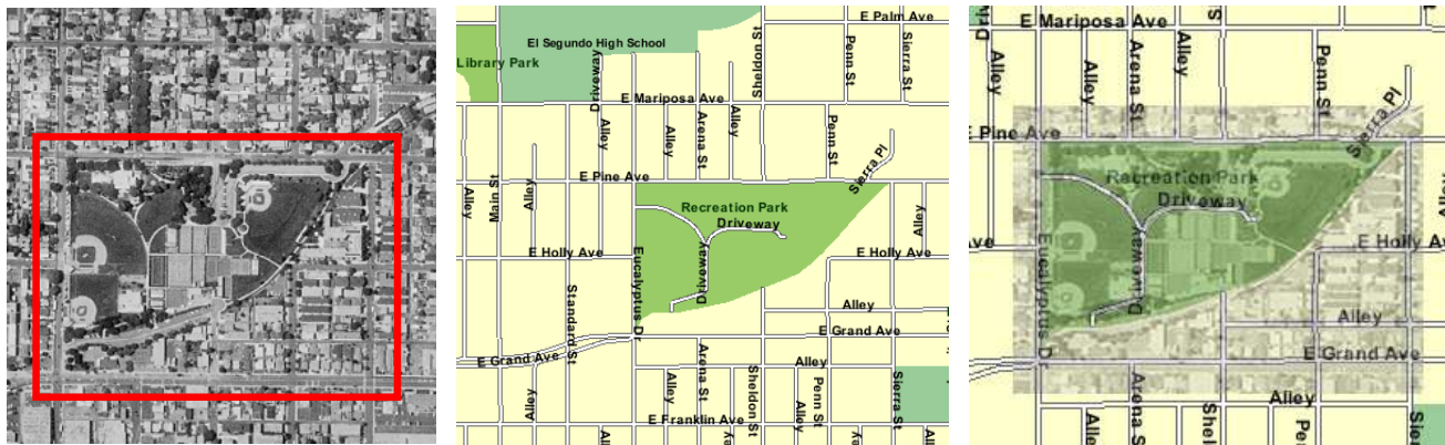
a) Orthoimagery with the area of interest highlighted b) ESRI street map (whose geo-coordinates are unknown) c) Imagery with aligned map
