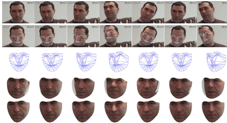
Fig. 6. Example of the output of the AAM tracking and the associated shape and appearance features: (Top row) the original sequence, (Second row) the AAM tracked sequence, (Third row) the similarity normalized shape features (SPTS), (Fourth row) the similarity normalized appearance features (SAPP), (Bottom row) the canonical normalized appearance features (CAPP).
