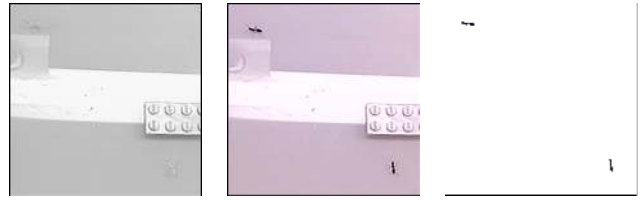
Figure 7: Use of background differencing to find moving objects. Left: Background image computed using a running locally weighted average. Center: Sample “live” image. Right: Difference between background and live image reveals the locations of two ants.
