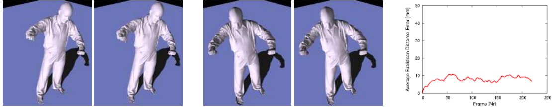
Figure 6: (left) Two pairs of images comparing the input (left sub-image) to our skeleton-based result (right sub-image). In either case the renderings are visually almost indistinguishable. (right) Plot showing the low average Euclidean distance error between input and reconstructed vertex positions for the human-sized model.
