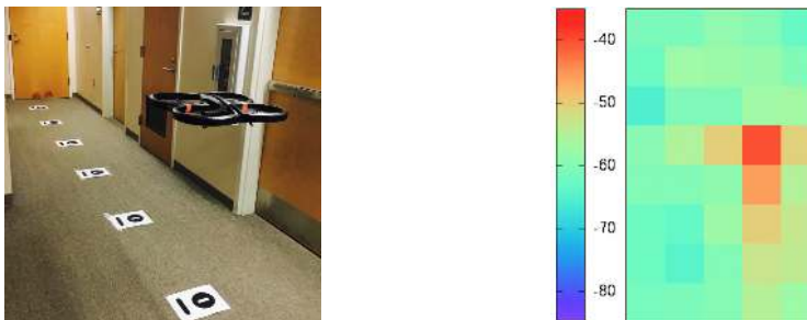
Figure 1: Drone in flight, visualization of wireless signal strength (dBm)
