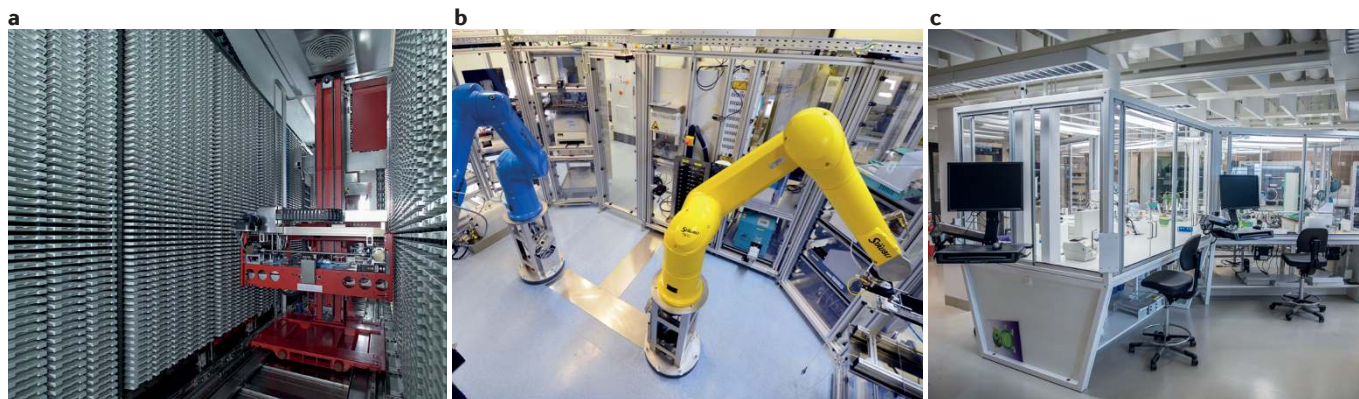
Figure 2 | Automated drug discovery facilities. a | Millions of compound samples are stored in compact high-capacity facilities and handled by robots. b | Robot systems perform both high-throughput and medium-throughput screening of up to ten thousand samples per day to determine the activity against the biological target of interest. Multiple arms and flexible workstations enable fully automated liquid dispensing, compound
