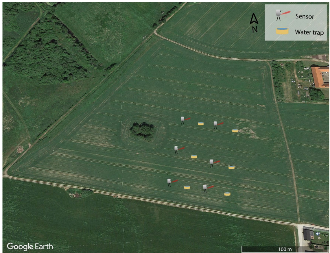
Figure 7. Layout of sensors and traps on the field. Sensors and traps were placed in a grid pattern ca 30 m from the field edges. The four north–south transects are separated by ca 22 m and consists of either sensors or water traps, spaced by 45 m. Image data from Google Earth 2021, Aerodata International Survey Mapdata 2021.
