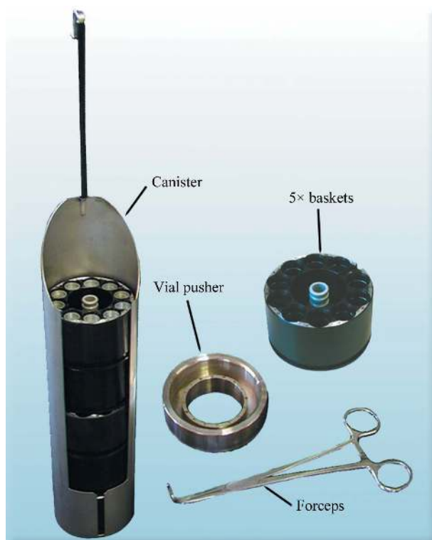
Figure 7 The SC3 Starter Kit which consists of five SC3 baskets, a vial-release tool, a forceps or basket handler and a canister to transfer the baskets with a dry shipper.
