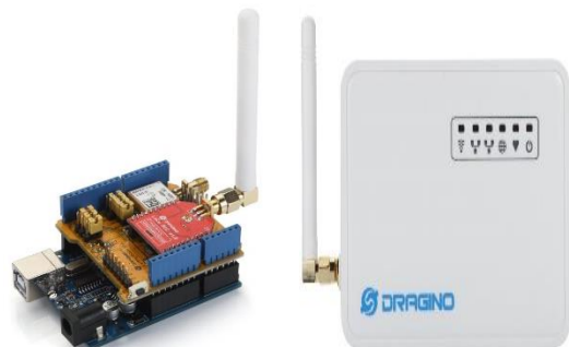
Fig. 5: LoRa Shield with Arduino UNO and Gateway
