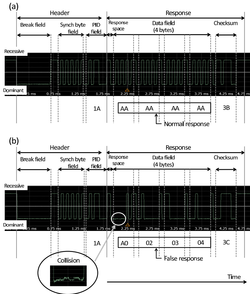
Fig. 9 Experimental results of waveform of header and response transmitted in the bus. (a) Waveform of message frame in normal communications. (b) Waveform of message frame in communication when attack is performed. Collision occurs at the first byte and a false response is transmitted to the bus after the collision.
