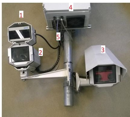
Figure 5. Roadside ITS station sensor system. From left to right: Laser scanner (1), NIR camera (2), IcOR stereo camera system (3), roadside unit PU (4) and air temperature sensor (5).
