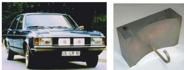
FIGURE 1. Bistatic 35 GHz pulse radar mounted in the front of a passenger car and view on one of the two parabolic antennas [26]. Left photograph: Telefunken, courtesy of H.H. Meinel; right photograph by W. Menzel.
