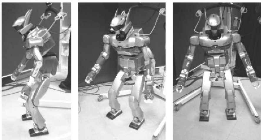
Fig. 8. Postures generated on an HRP-2 humanoid.
