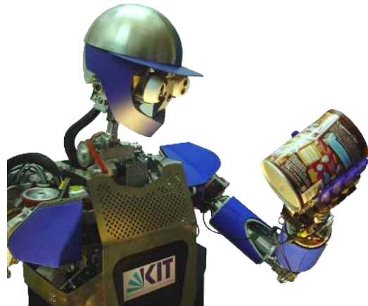
Fig. 1. The proposed approach allows to acquire representations of objects held in the hand of ARMAR-III.
