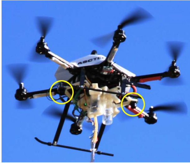
Figure 4.13: Ultrasonic sensor placement.
