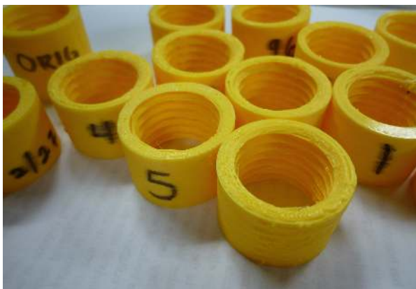
Figure 4.5: Several test vial thread jackets printed to find the best fit.
