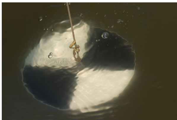
Figure 3.1: Secchi Disk for measure water opacity. Image courtesy of White Lake Stewardship.
