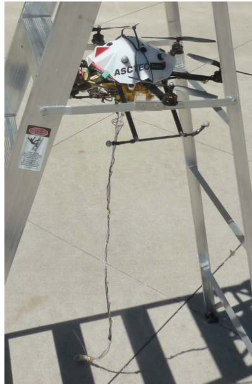
Figure 6.2: UAV at fixed altitude for pressure characterization.
