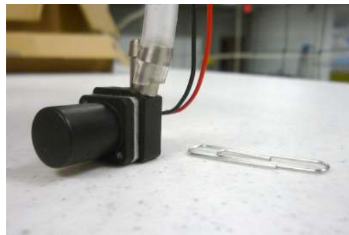
Figure 4.7: Micropump with reference paperclip.
