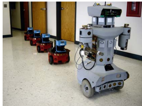
Figure 1. Four relay robots convoying behind the lead robot (laboratory demonstration scenario).
