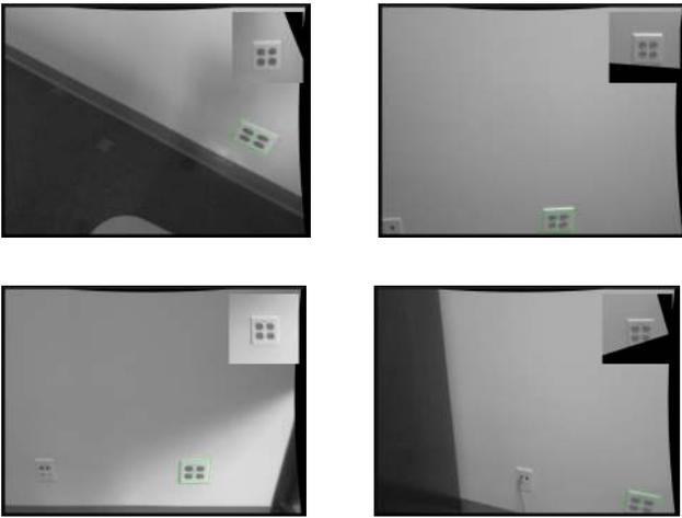
Fig. 7. Outlet detections with varying pose, illumination, and partial occlusion. The resulting rectified outlet patch is also shown.
