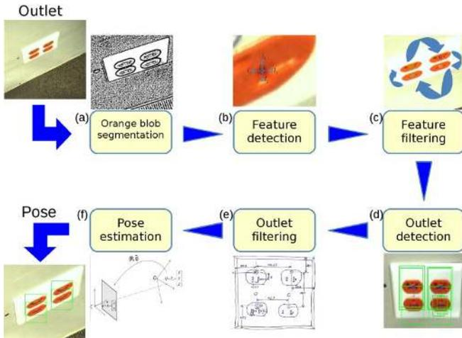
Fig. 8. Processing flow chart for finding outlet pose.
