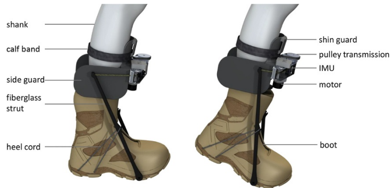
Figure 1 Autonomous leg exoskeleton. The posterior protrusion of the device was reduced compared to the former exoskeleton [6] by using shorter struts and increasing the length of the heel cord. Further, side guards were added to eliminate strut rubbing against the calves during walking.
