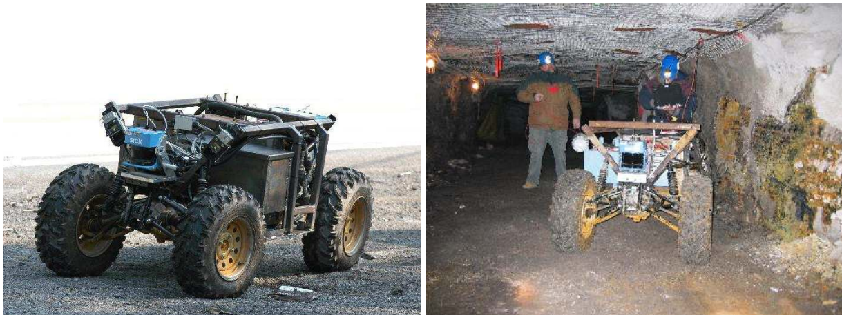
Figure 1: Left: The Groundhog robot is a 1,500 pound custom-built vehicle equipped with onboard computing, laser range sensing, gas and sinkage sensors, and video recording equipment. Right: Testing the system inside the Bruceon Research Mine, a well-maintained mine accessible to research teams.
