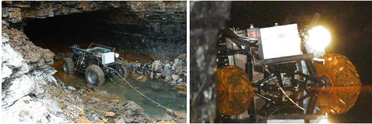
Figure 2: On October 27, 2002, Groundhog was deployed into the Florence mine near Pittsburgh, PA. This experiment is a first in a series in which the robot navigates an environment inaccessible to people, but still under remote control.
