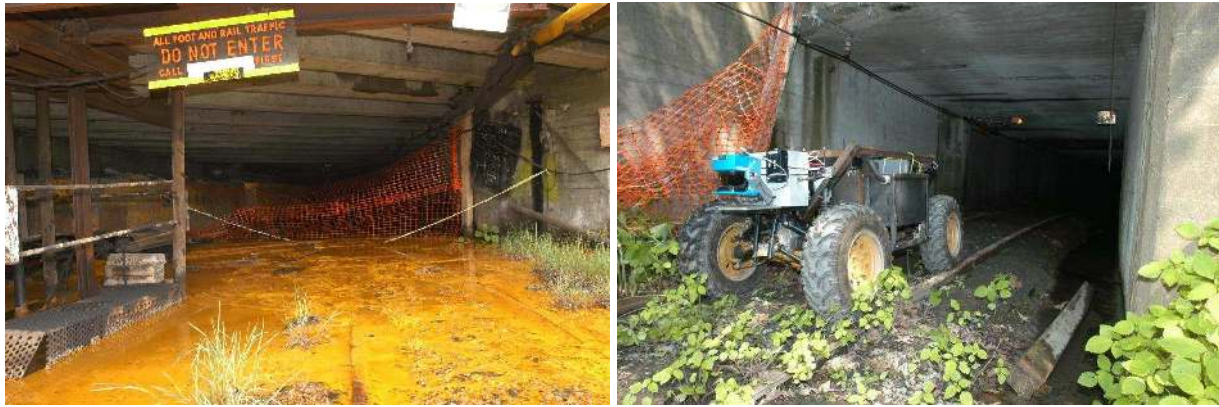
Figure 3: On May 30, 2003, Groundhog enters the Mathies mine near Courtney, PA. For the first time, Groundhog operates in fully autonomous mode, beyond the reach of our wireless communication link. It autonomously descended 308 meters into the mine before making the correct decision to turn around after sensing a non-negotiable ceiling beam draped diagonally across the robot's path. These photographs show the two entrances to the mile-long corridor system.
