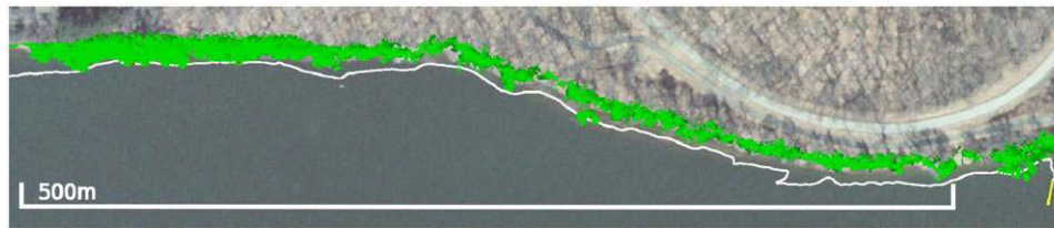
Figure 17. Satellite image with overlaid flight trajectory (white) and bank map (green point cloud) collected from a 660 m autonomous flight over water along the bank of a lake.
