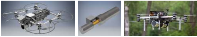
FIGURE 22. A new platform under development that uses fire-extinguishing capsules as projectiles. The first two photos on the right show 3D render of the platform and launcher design, photo on the left shows constructed platform.
