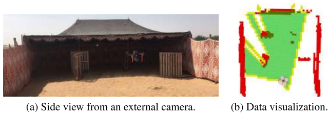
FIGURE 16. Experimental verification of the indoor motion planning and exploration techniques in the desert near Abu Dhabi, United Arab Emirates before MBZIRC 2020. In the image on the right, the red blocks denote obstacles, the green blocks show the already scanned space, and the yellow blocks denote frontiers for exploration. A video from this experiment is on YouTube 12 .
