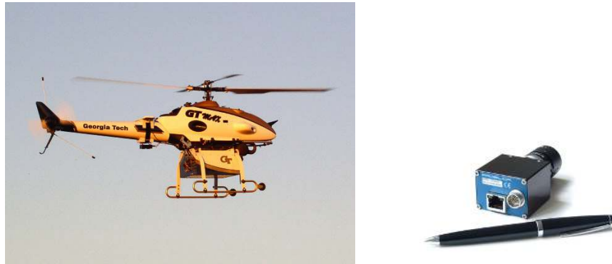
Figure 11. The GTMax rotorcraft UAV is a modified Yamaha R-Max helicopter equipped with custom avionics. For testing the vision-based algorithms, a machine vision progressive scan camera is used for acquiring images. Two onboard computers divide up the tasks of image processing and estimation.
