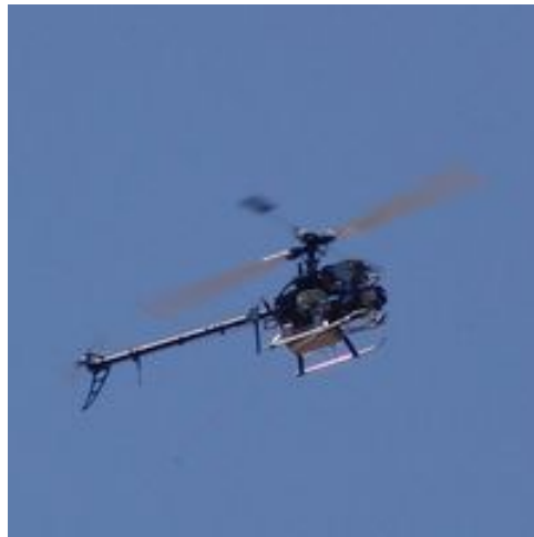
Figure 1. Small unmanned aerial vehicles, such as the GTFirstResponder UAV shown above, are often not capable of carrying large computer systems. A monocular downward facing camera is a typical payload on such UAVs.
