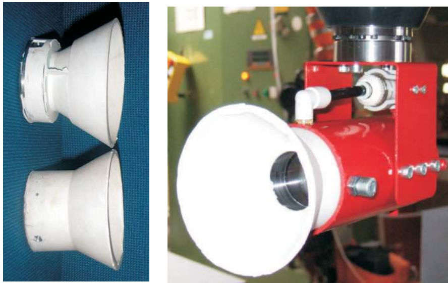
Fig. 3. Left: two examples of silicone gripper; right: gripper mounted on robot with camera inside
