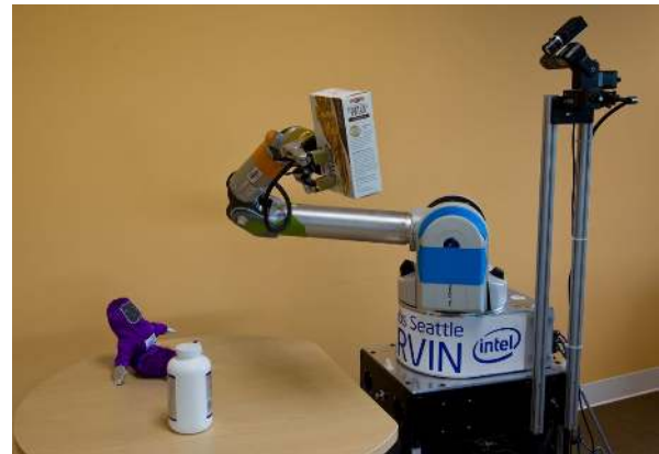
Fig. 1. Experimental platform. We used a WAM arm with BarrettHand on a Segway base. Mounted next to the arm on a pan-tilt unit is a depth camera.
