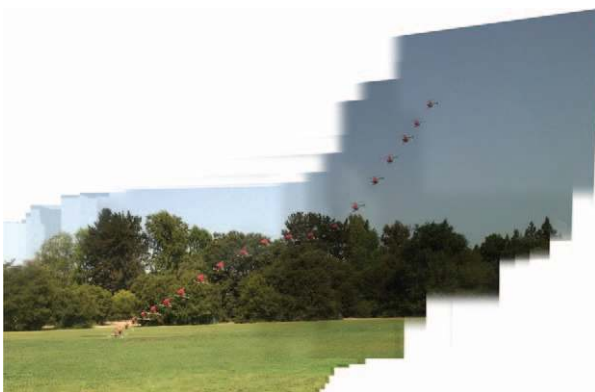
Fig. 13. Mosaic of one of our autonomous auto-rotation flights as viewed from the left of the helicopter. (Sampled at 4 Hz.)
