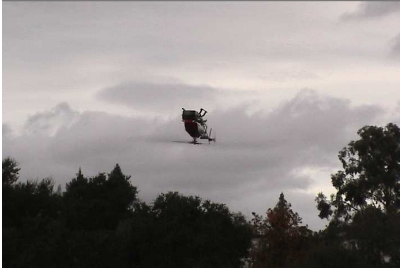
Fig. 3. Helicopter in autonomous sustained inverted hover.
