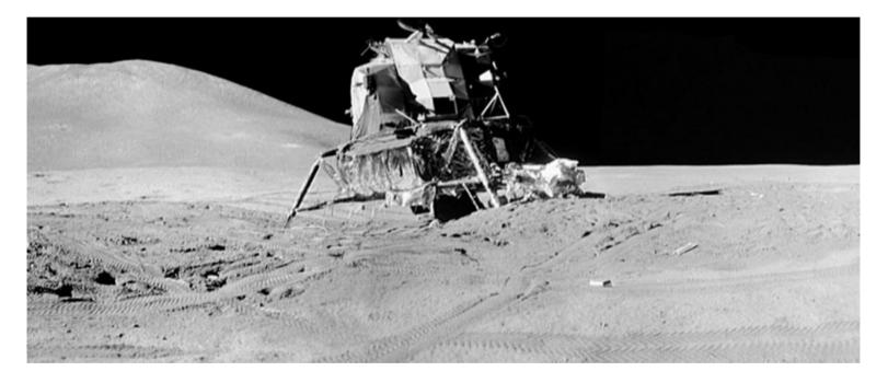
Apollo 15 set down on the rim of a small crater, damaging the engine bell and tilting at  $\sim 10^{\circ}$
