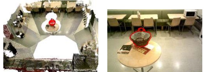
(a) Meta-Room (RGB) and segmented dynamic cluster (red). (b) Camera image containing segmented cluster and mask (red)
