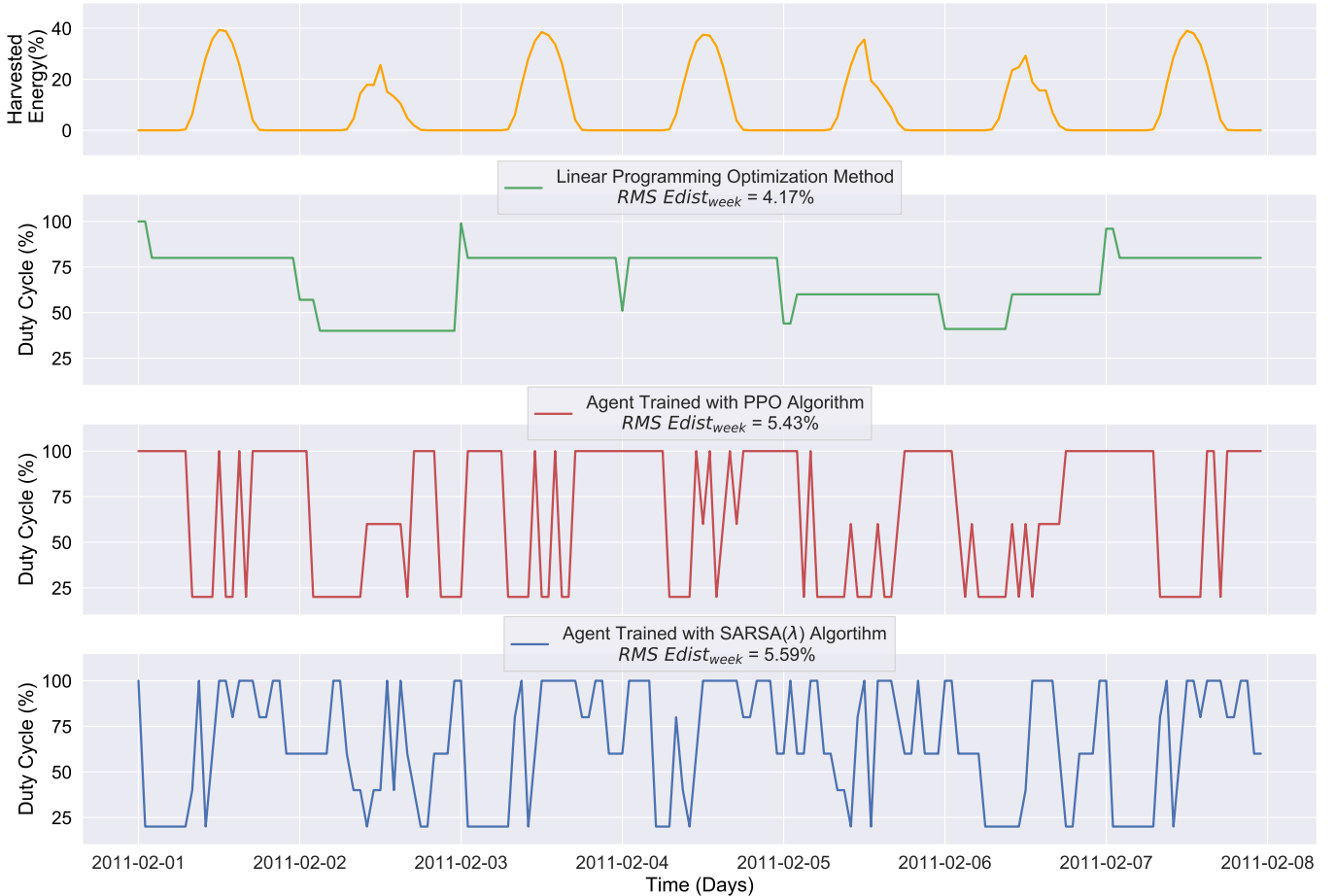
Fig. 3. Comparison of PPO policy to SARSA( \lambda ) and offline policy for a week of Tokyo 2011
