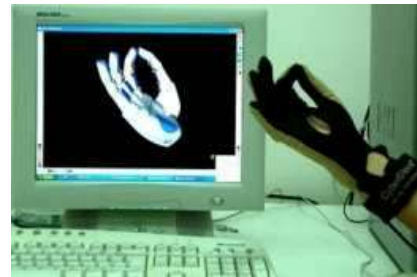
Fig. 6 Human hand with the sensorized glove connected to the mechanical hand simulator.
