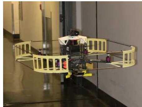
Fig. 1. The experimental platform with onboard computation (1.6 GHz Atom processor) and sensing (laser, camera, and IMU).
