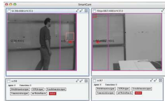
(b) Handover to camera B: the person is in the migration region (red square).
