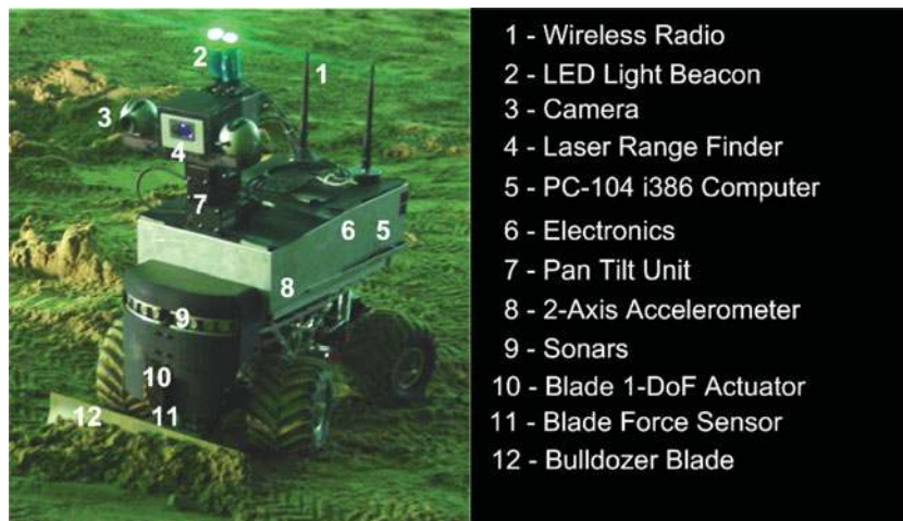
Fig. 26. An Argo robot equipped with a 1-DoF bulldozer blade, a laser range finder, a pair of Logitech® Quickcams™ affixed to the pan-tilt unit and an assortment of other sensors.
