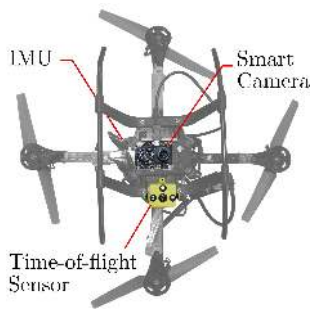
Fig. 1 Bottom view of the ASCTEC Hummingbird quadrotor used in the experiments. The vehicle is equipped with a built-in IMU, a smart camera and a time-of-flight range sensor.
