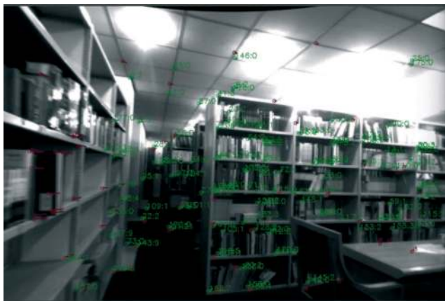
Fig. 6. An example of an image of the stereo camera during the experiment in the library. The numbers represent tracked feature statistics that are used to decide whether to keep or discard the feature.
