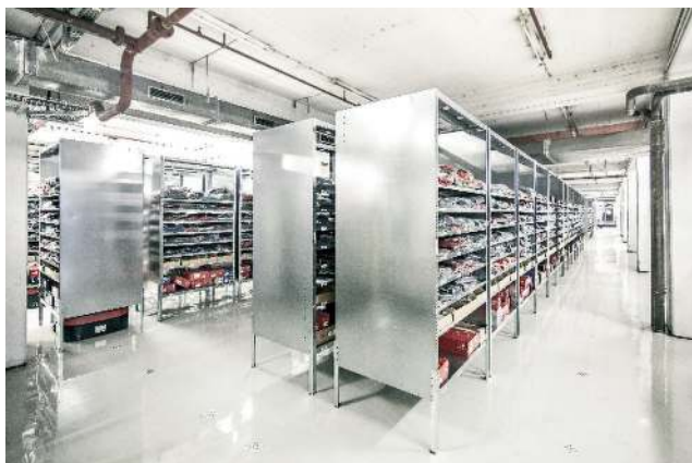
Fig. 1. SafeLog partner Swisslog’s automated CarryPick system
