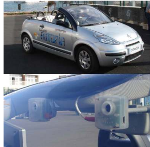
Fig. 1. Experimental vehicle and the onboard stereo sensor.
