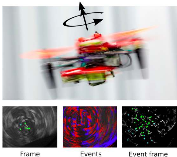
Fig. 1: Controlling a quadrotor with complete failure of a rotor causes fast yaw rotation, over 20 rad/s (top figure). Bottom figures show a standard frame and events captured by an onboard event camera. Bottom Left : standard frame with motion blur. Bottom Center : Events only (blue: positive events, red: negative events). Bottom Right : Event frame generated from events. Blue circles are detected features, green dots indicate tracked features.
