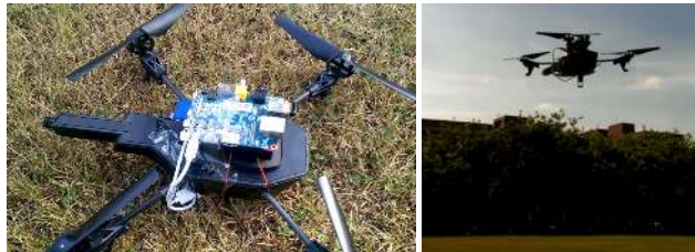
FIGURE 11. The parrot AR. Drone with our attached single-board computer for online processing.
