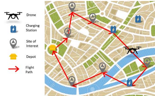
Fig. 1. A drone flight mission plan with charging stations.
