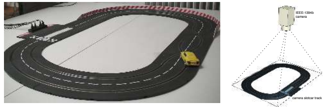
Fig. 1. The visual slot car racer task. The controller has to autonomously learn to steer the racing car by raw visual input of camera images.
