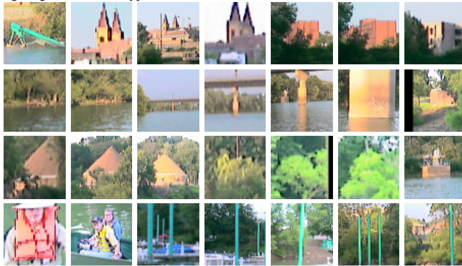
Figure 7 Some sample color blobs extracted during a test run on the river. These correspond to: the dock support poles, boat covers, buildings, lifejackets, distinctive trees and stumps, bridges.
