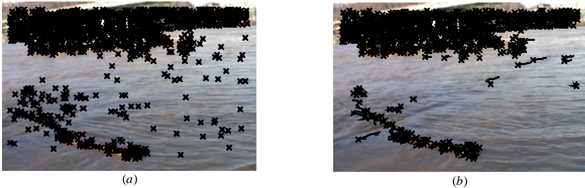
Figure 1 (a) The 1000 top features detected using a typical corner detector. Some but not many are detected on the water surface. (b) After tracking for one second at 10 frames per second most of the water features are lost whereas features on the land and a foreground object maintain track. While the camera has not moved, the water features have shifted considerably. In this example the detector and tracker used is that by [1] and it shows similar ability to exclude water surface features to our optical flow algorithm.
