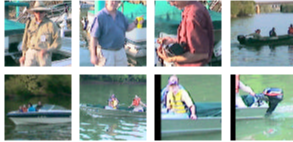
Figure 8 Some sample motion blobs extracted during a test run on the river. These correspond to people walking in front of the camera while still docked, and passing boats seen while traveling on the river.
