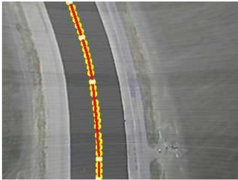
Fig. 2. Our Second vision-based UAV navigation tracking a canal [8]: The experiment was done on a canal stretch of around 700 meters.
