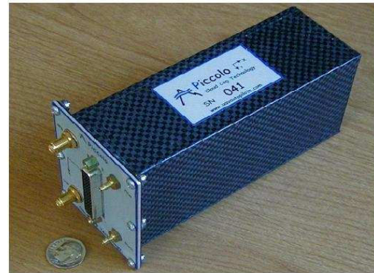
Fig. 9. Piccolo avionics package that performs low level flight control and stabilization.
