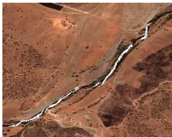
Fig. 12. Coordinates of the river estimated from the vision algorithm during the exploration shown with the map of the Camp Roberts river.
