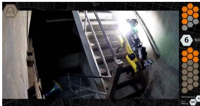
Fig. 1: Live-mission image of Autonomous Spot robot climbing down four flights of stairs in the Urban Circuit of the DARPA Subterranean Challenge. This platform is one of the elements in team CoSTAR’s solution that won the Urban Circuit of this competition. (Image credit: DARPA).
