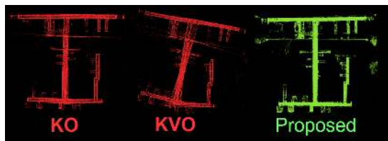
Fig. 7: Map created by Au-Spot while exploring an office building at NASA's JPL with different odometry sources: KO (left), KVO (middle), and the Proposed method (right).
