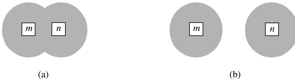
Figure 3-3: Region of dependency for \mathbf{G} vectors. (a) Sensor footprints of cells m and n overlap - \mathbf{G}^m and \mathbf{G}^n are dependent. (b) Sensor footprints do not overlap - \mathbf{G}^m and \mathbf{G}^n vectors are independent.
