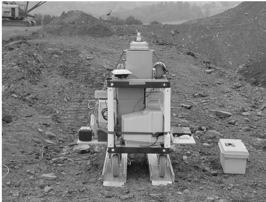
Figure 5-1: Experiment Platform. The brass colored cube on top is the Z+F laser.
